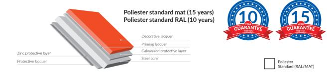
**Poliester Standard** - coated sheets are the most popular option for metal roofing. Currently, sheets that are double-side galvanised with anti-corrosive layer, priming or organic paint are used. The top layer provides the colour and texture, as well as protects against outdoor conditions.
